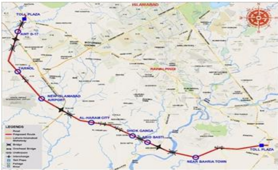
Figure 3: Alignment # 2 for the proposed Rawalpindi Bypass (51 Km)
